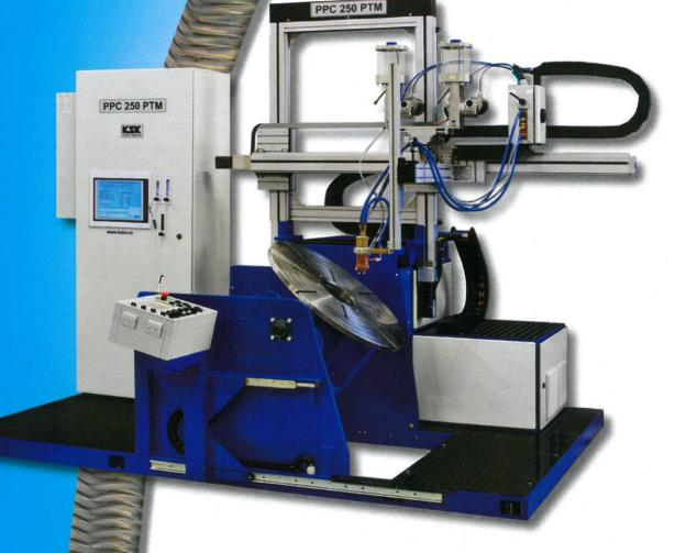
With hardfacing machine PPC 250 PTM it is also possible to hardface asymmetric shapes.
