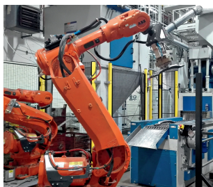
Robotic workplace equipped with robots for handling metal parts at high temperatures.
